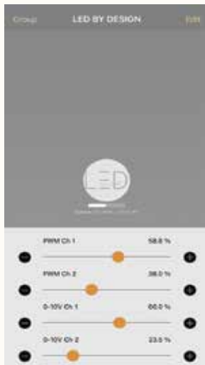
Control 4 Individual Channels 2 of PWM and 2 of 0-10V
