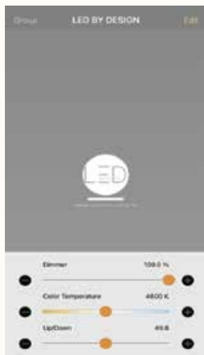
Control 2 set of Tunable white(TW) Example: direct and indirect light
